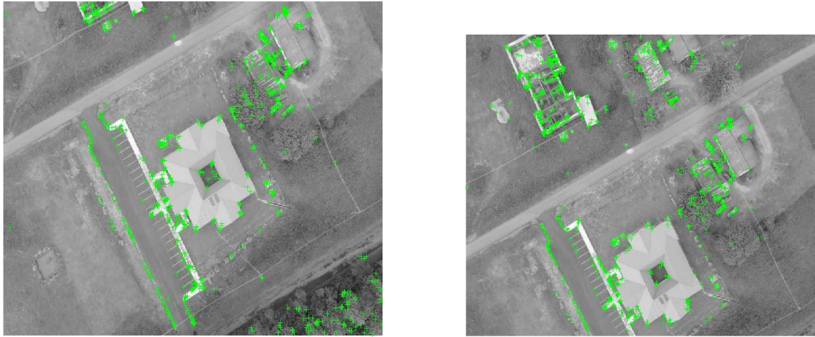
(a) Image 1 (b) Image 2 Figure 5.1 (a) and (b): Detected Features using BRISK on image1 and Image 2
